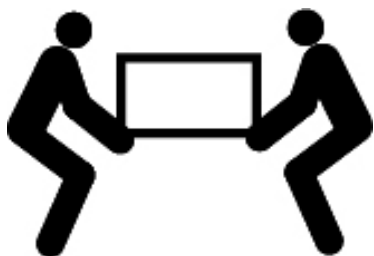
Figure 2-1. Lifting the centrifuge at both sides.
